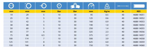
**RECOMMENDED FOR** Vacuum and pressure hose (SD) for transfer of fuel oil and other petroleum
