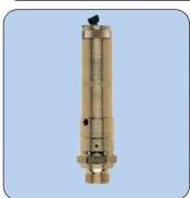
Safety valves serve to blow out non-poisonous and nonflammable gases into the atmosphere in order to protect pressure tanks against overpressure.
